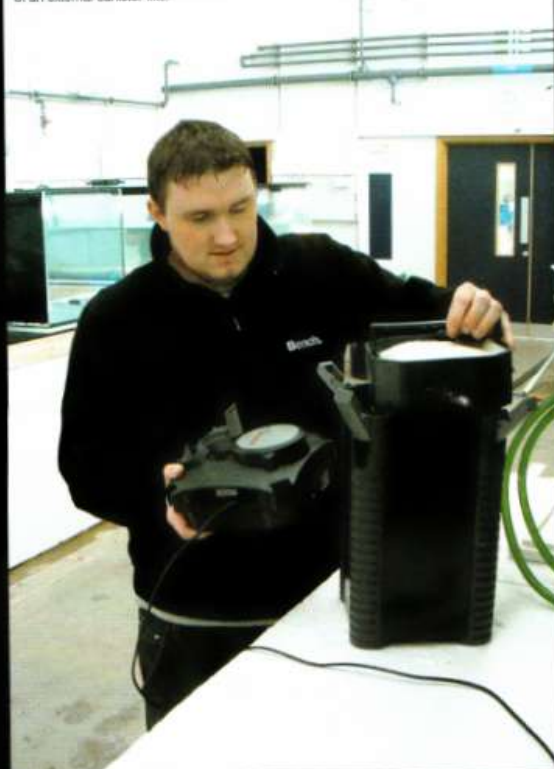
Swapping the internal compartments of an external canister filter
