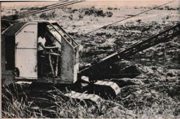
The dragline bucket digs out the banks between the pools so the pools can rotate their position annually, giving the pools fresh dirt which supports more life than washed out sand.
