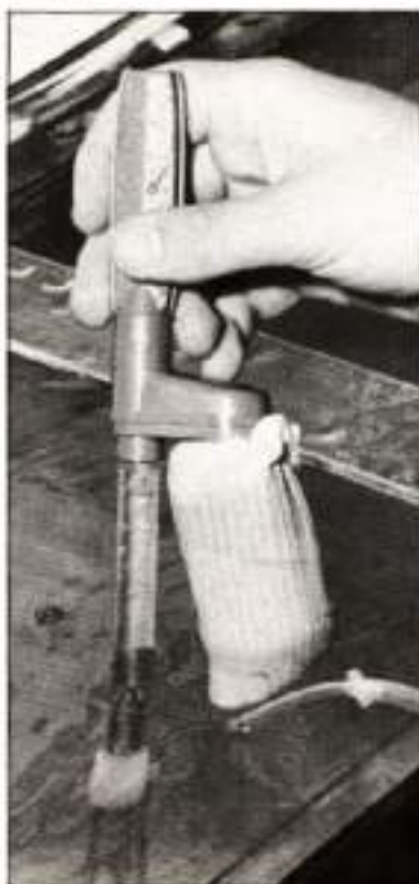
Step 11. USING an air pump powered vacuum cleaner like this gently remove the settled humus and algae from the filter bed. The cleaner is best for larger particles.
