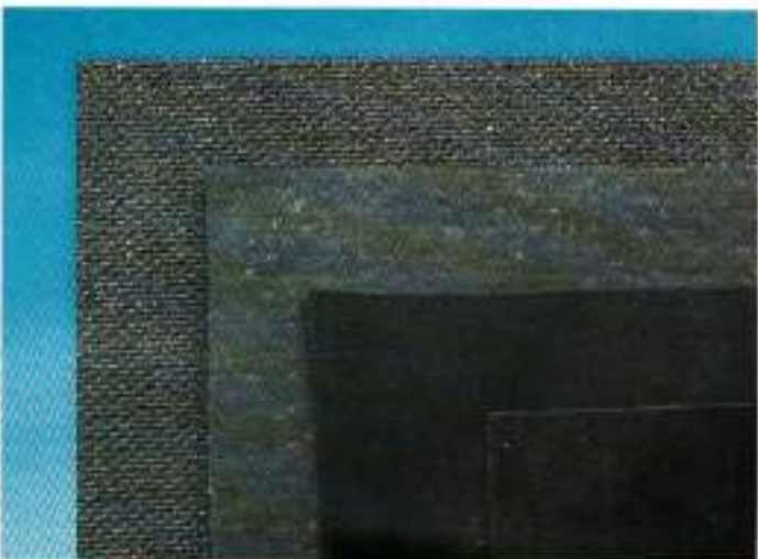
Liners from Reef, from outside in: Buryl 80/20; Buryl 75/20; DraktechnoFolie; Reifexfolie
