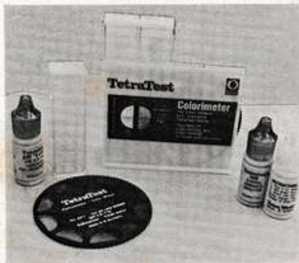
The TetraTest Colorimeter and water-testing reagents. A test colour wheel is shown, which can be inserted into the Colorimeter for use with the appropriate test solution.
