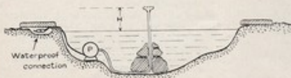
Sectional diagrams of ponds with submerged pump (P) are shown on this page. The working 'head' (H) for the pump is the vertical distance between the pond water surface and the water outlet (a cascade in the top diagram and a fountain in the lower diagram)
