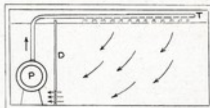
Arrangement of quarantine tank with high-power filtration unit. Water reaches the pump (P) through holes in the lower part of the plastic sheet D and is returned via the perforated pipe T.
