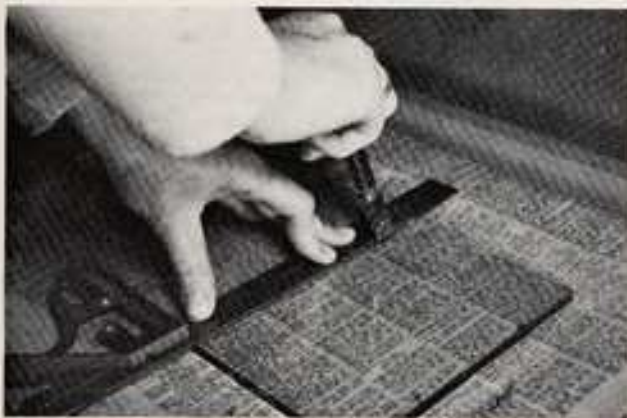
A confident approach to making the cut, plus a sharp cutting wheel, a straight edge and the glass supported on a soft pad (e.g. newspaper) produces results
