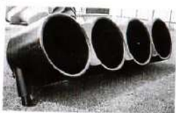
Centrifugal Filter System showing main 4" 1/2" head pipe and 2" discharge pipes from each compartment.
