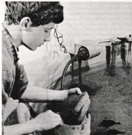
Detail of the filter assembly, showing the pump and heaters in the background. Polyethylene sponges are used to filter solubles from the water and to trap floating oil that cascades into the filter through the slits in the filter container that extend above the water line.
