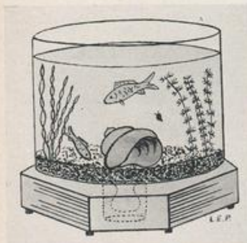
New use for a glass sandwich cover. The method of recessing the plinth to take the knob of the glass is shown in broken lines
