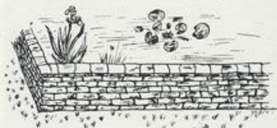
A raised pond made with walling stone and floated over inside with concrete
