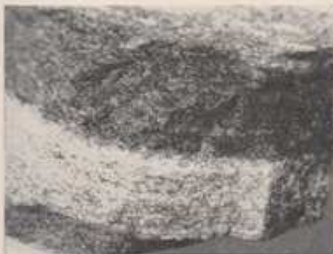
Biotite gneiss (Sutherland), slightly enlarged. A thin-banded gneiss material in which the banding is caused by black mica (biotite)
