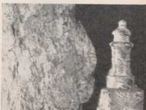
Serpentine (Cornwall), three-quarters natural size. Mottled in light and dark green, the specimen's texture is such that it splinters readily. The serpentine lighthouse has been turned and polished.
