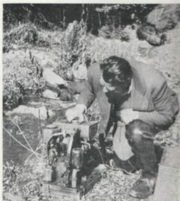
Electricity-generating motor in use by the Kostina river for the capture of trout alive after electric "stunning"
