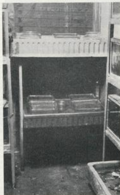
Two old-fashioned sinks in use as thermostatic baths for the fish containers.
