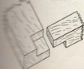
FIG. 3. A HALVED JOINT
