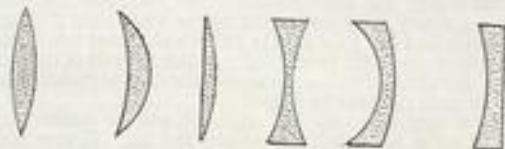
Shapes of various lenses used singly or in combination in modern microscopes
