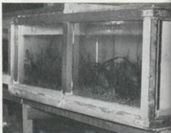
One of the wooden-frame aquaria used by Mr. Rusbridge, showing the metal brackets used to strengthen the corners
