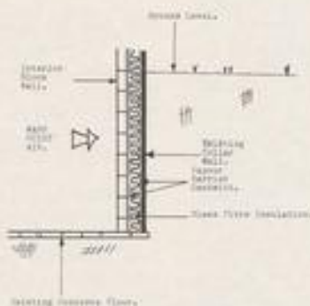
FIGURE 1. Section of wall construction to provide insulation.
