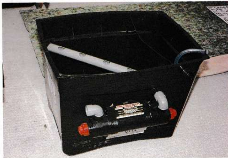
External filter with aeration on input, UV on output.
