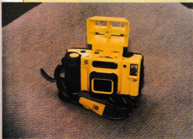
▼ Underwater compact camera with sighting device attached.
