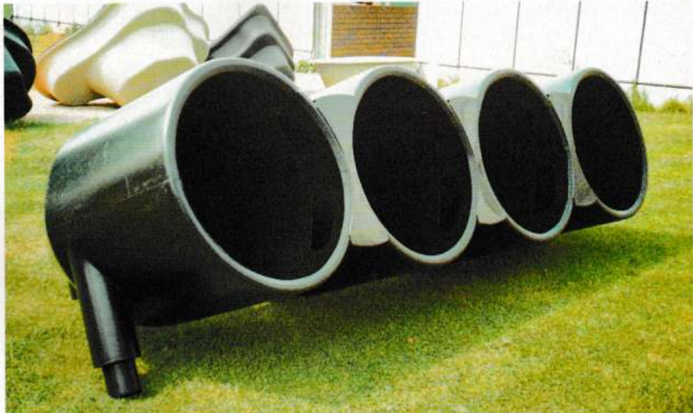
A centrifugal filter system showing transfer ports in each chamber.
