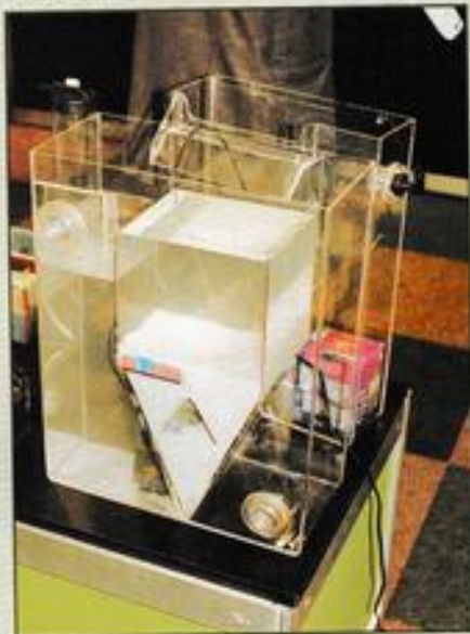
BELOW THE SPECIAL SILICA SAND FILTER MEDIUM IS MOVING IN THE WATER ALL THE TIME. Photo: A&P Library
