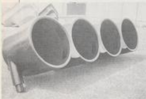
Centrifugal filter system showing transfer ports in each chamber.
