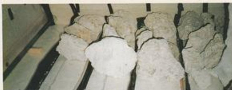
Construction of the back wall (tank is lying on its side). The Faxa Limestone blocks can be seen resting on their appropriate sections, with black tape in between (see text for details).
