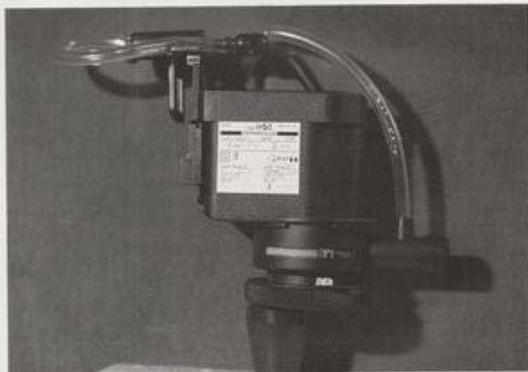
This powerhead has many operational features: a variable flowrate (in the conventional direction only), a reversible flow for use where 'reverse flow' undergravel filtration is preferred, swivelling directional return tube, filtered air intake on the aerating venturi and a choice of tank mountings.
