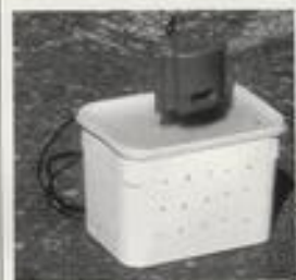
Powerheads are versatile pieces of equipment. In this case, I used it to drive a small experimental pond filter.
