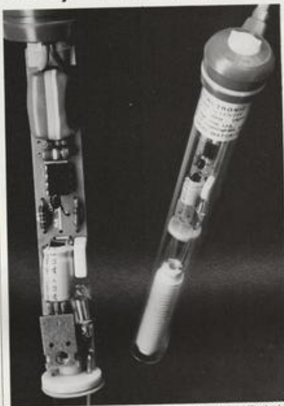
Most thermostats work on the bi-metallic strip principle. The 'strip' can be seen at the bottom of this unit (it has a hole).
