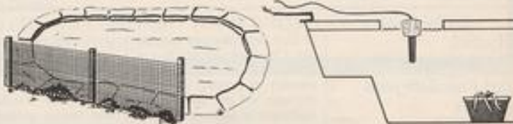
Top, despite appearances, life ticks on, slowly, under ice and snow. Above left, a temporary fine mesh fence to catch leaves on the prevailing wind side of the pond. Above right, low voltage pool water heater keeping small area free of ice. On contents page, high tensile strength fishing line stretched across the pond can deter predatory birds.
