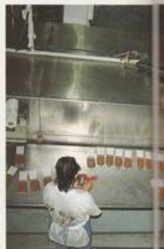
Part of the production line during the filling and freezing (note the freezer tunnel) of one of the 'formula' foods.
