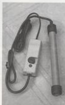
The in-line controller with this aquarium heater maintains the correct temperature in association with the sensing device built into the heater itself.
