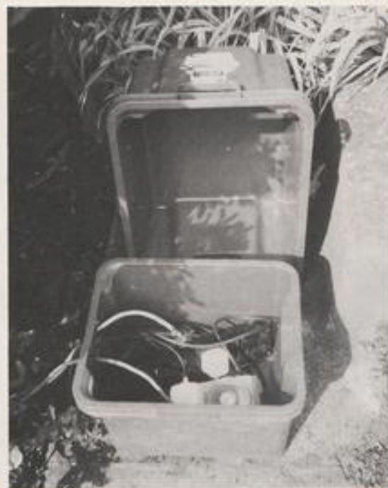
Dr Ford's home-made waterproof electrical fittings protector, as featured in the July article referred to by Dave Lunn.
