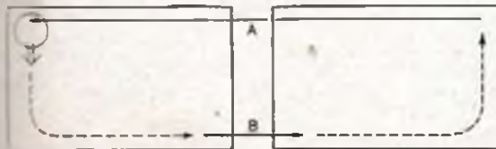
Fig. 1. Small circulating system using the author's suggested arrangement of two tanks and two syphons (A and B).
