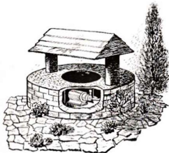
There are several ways of concealing the pump used in a water garden. Here it is placed in an ornamental well head.
