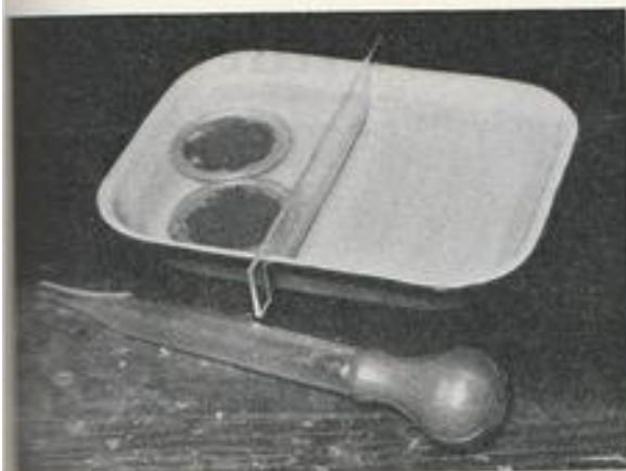
Apparatus required for the "pan method" of culture: a strip of Perspex across the enamel dish separates two feeding rings from the brine on the other side
