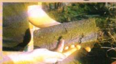
1. The problem - pre-filter sponges clog quickly with an ugly muck and slime
