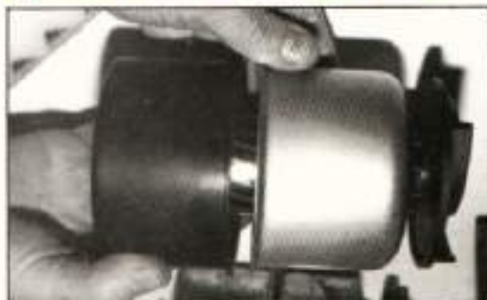
The wear casing of the pump is a push-fit, incorporating a sealing ring (not shown).
