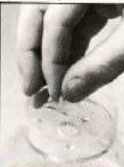
Unscrewing the cover to the pouring hole in the base of the plexiglass inner container. The air hole for the gas generated is visible to the left.
