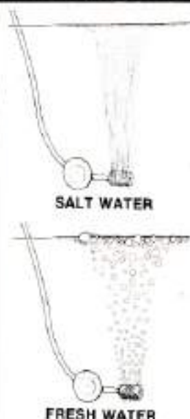
An airpump delivering identical volumes of air will give a much finer stream of bubbles in the dense water of a marine aquarium (top) than in fresh water. It's quieter, too!
