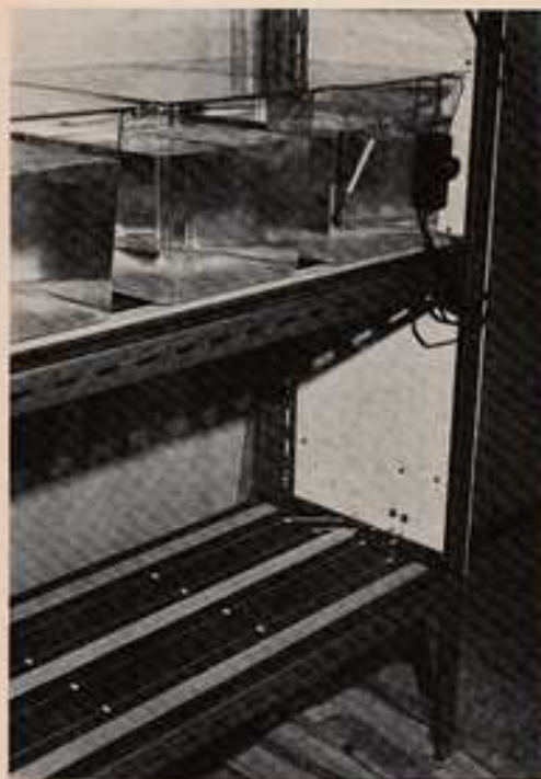
On the lowest shelf of this staging constructed by Mr Dave Ellis (British Killifish Association) the parallel arrangement of the lengths of electric blanket heating cable is shown. Plastic tanks on the upper shelf are supported above similar low-wattage cables.
