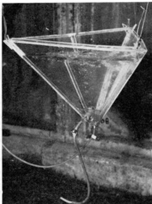
The author's brine shrimp hatcher, made from three triangular pieces of Perspex
