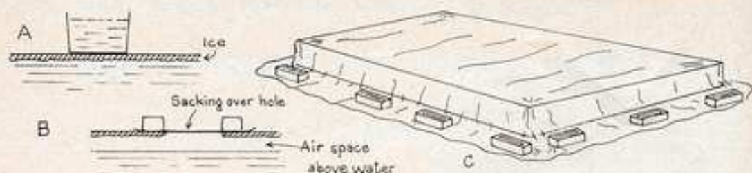
To avoid trouble during freezing spells use a can of boiling water to make a hole in surface ice (A), remove some water and cover the hole (B) or cover the whole pond with a frame and plastic sheet (C)
