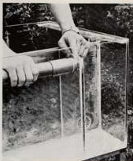
Compartment A is on the right with the water entry point seen at the bottom. The perforated 'streaming tube' is being fitted in compartment B.
