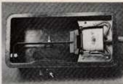
A typical medium-priced diaphragm-type aerator with the base removed to show the arrangement of the vibrator arm, diaphragm and valve block. The arrow indicates the position of the air control.
