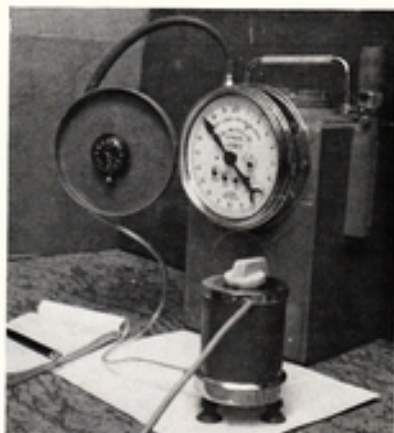
The Perma (in the foreground of the picture) on the PFM test bench during measurement of its air output by meter
