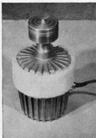
The fountain-only form of this new Sealion submersible pump has an 85-hole jet that can produce a four-tier pattern of spray 8 ft. high and 7 ft. in diameter
