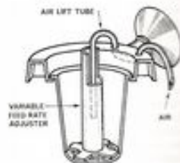
Cut-away view of the Feeder
