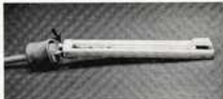
An internal thermostat removed from its glass tube for adjustment of the temperature setting screw shown by the arrow
