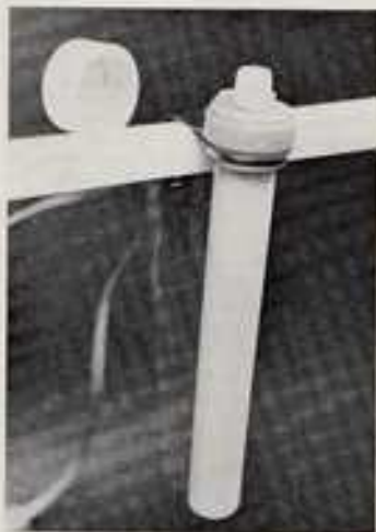
Internal thermostat of non-submersible design (Kens), with the top cap removed to show the temperature control. This particular instrument is cased in a shatter-proof material, not glass, and has a metal strip for attachment to the tank frame.
