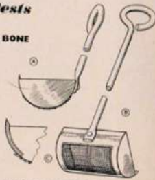
a=side view, b=underside view with the gauze soldered in position, c=sectional side view showing razor-sharp edge.
