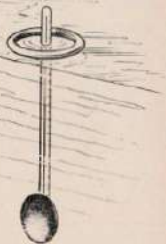
Perforated feeding rings may be fitted to the thermometer by means of a small nylon loop. —W. STOLT, Annecy, France.
