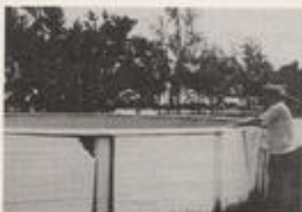
In the second stage of preparation, the filtered sea water is chlorinated with commercial bleach in a huge above-ground swimming pool. The final preparatory stage will be dechlorination 24 hours later with sodium thiosulphate (photographic hypo)
