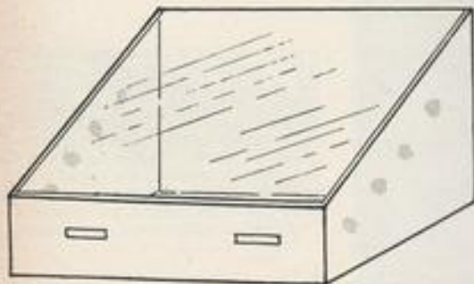
Writing-desk type of vivarium. The top glass sheet slides upwards to provide access to the case.
