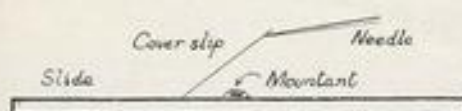
Side view of microscope slide bearing mountant with the object, showing the method of arranging the cover slip before lowering it gently over the mountant
