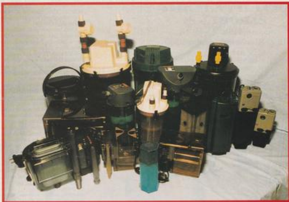
A collection of power filters. There are at least a dozen makes here, but all are effective because it is the bacteria that do the real work; the power filters merely pump water.
