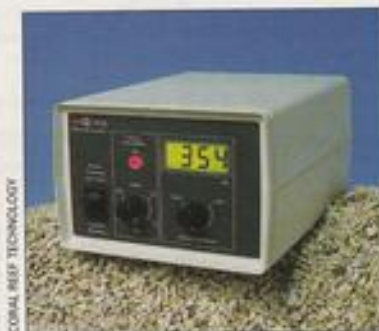
Ozone penetration can be combined with a redox control unit, as in this model, for optimal efficiency.
