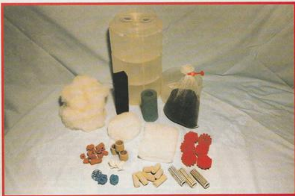
The plastic basket from a typical external power filter with media that can be used. From left to right, from the top: nylon floss, polyester wool, polyfoam square and cylinder, carbon (in a nylon bag), ceramic daisies, ceramic cylinders, nylon bag, polyball tubes, two colours of polyball interlocking pieces, sintered glass and plastic hair rollers. Use any, some, or all!
