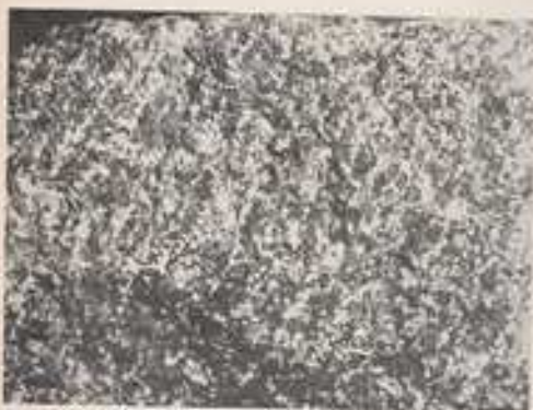
Fig. 2. Biotite granite (Aberdeenshire). Coarse-grained but of fairly even texture; clear quartz, whitish feldspar and abundant black mica (biotite) make up this specimen ( \times 24 )
