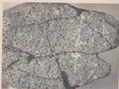
Fig. 1. Vesicular basalt (Argyle). The fine-grained structure is due to the quick chilling of the original molten magma. Tiny holes resulted from steam or gas in the cooling material ( \times 24 )
