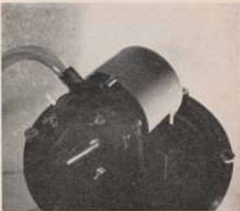
Closer view of the compact electric pump (220 volt, 28 watt) mounted on top of the filter unit
